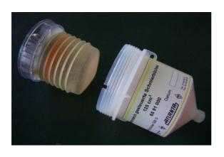
Using a suitable tool, push out the piston from the grease cup
