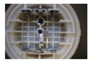
Fit the lid with the circuit board mounted onto the pressure chamber. Make sure that the contact surface on the underside of the circuit board rests on the contact spring in the pressure chamber. Slightly press the lid until the circuit board engages in the pressure chamber.
